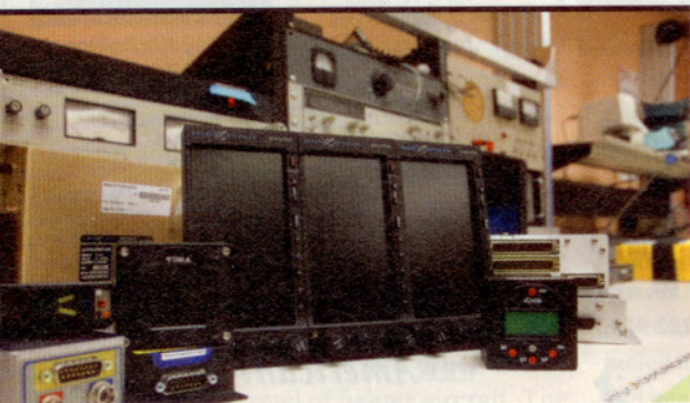
THE NEW PANEL will be dominated by Aspen Avionics' three-screen, Evolution 2500 display system.
